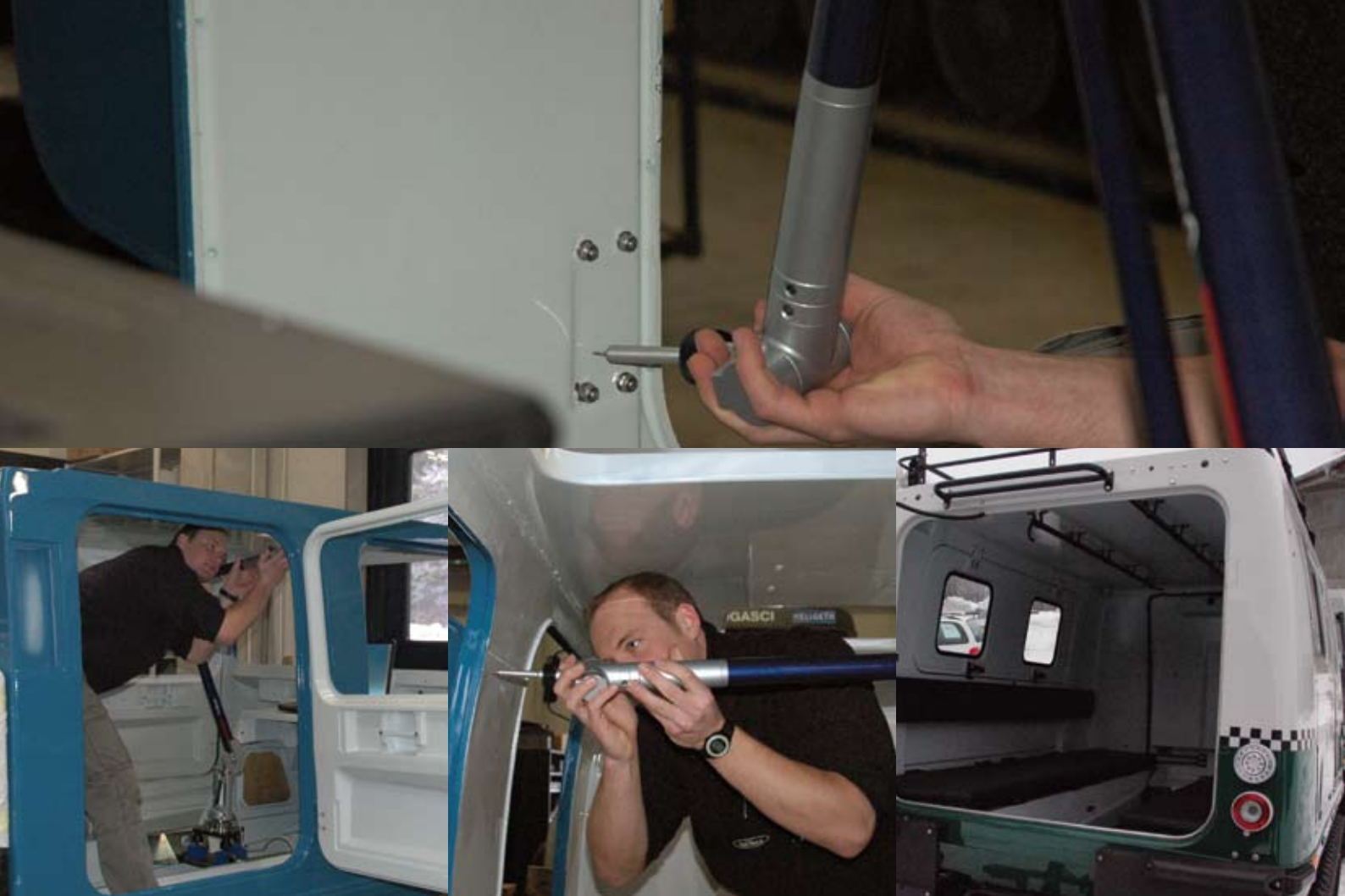
From empty cabin to finished converted transport vehicle. The typical ROMER flexibility allows you to measure the installation space inside the chassis.
